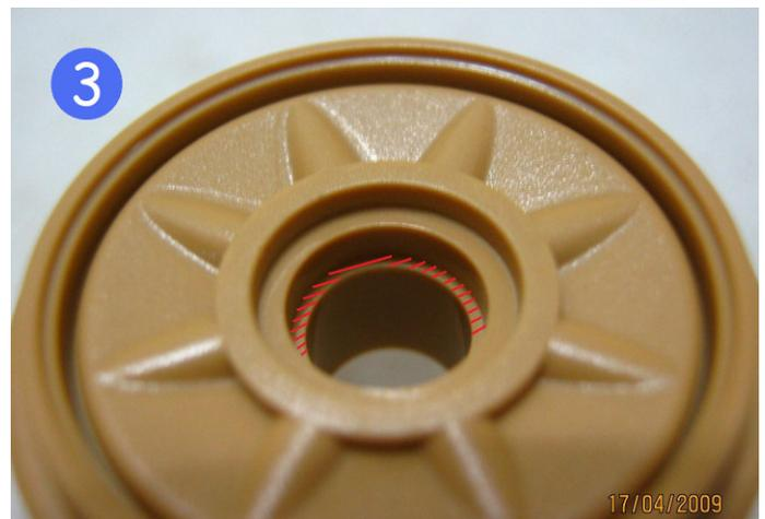
4 One method to rework the depth, is by using a 7mm drill bit.
