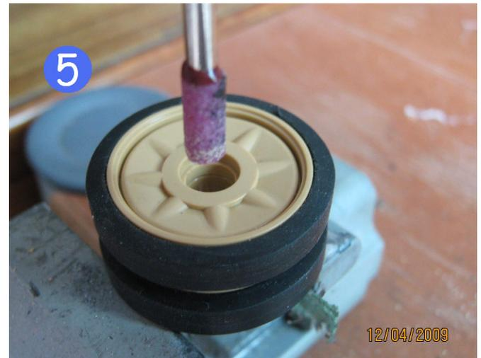
6 When 740 bearing is sitting in flush to the wheel, the rework is completed.
