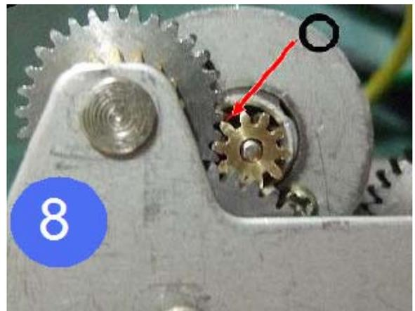
**9** With one hand holding the TU, and the other hand's thumb, rotate the motor pinion gear. The pinion gear must be able to rotate freely and smoothly. If rotating was fine, all screws can now be tightened. It will be good to apply some liquid thread lock to the screws, as it will ensure the Motors and Motor Assemblies will stay firmly in place.
