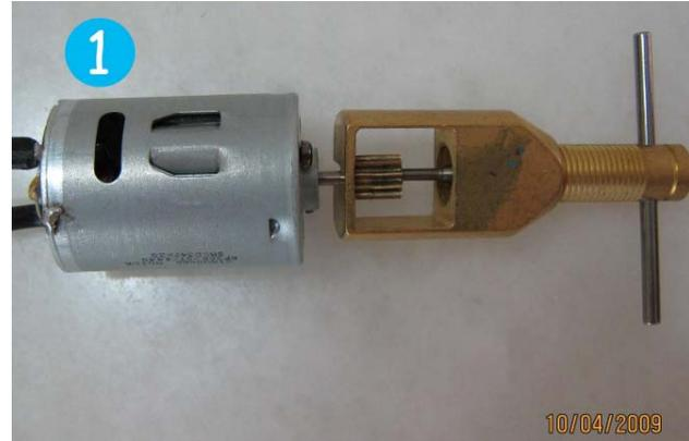
2 The pulled out 10T Pinion Gear **cannot** be re-used again.
