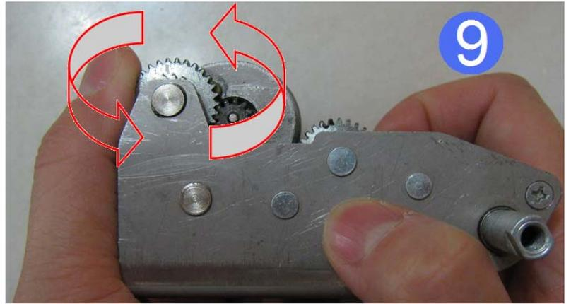
**10** If the pinion gear is not rotation smoothly, the motor position will need to be moved away from its adjacent gear. As shown, direction of motor's position will need to away from **X**. This is a usual case if the pinion gear is not a 10teeth type.
